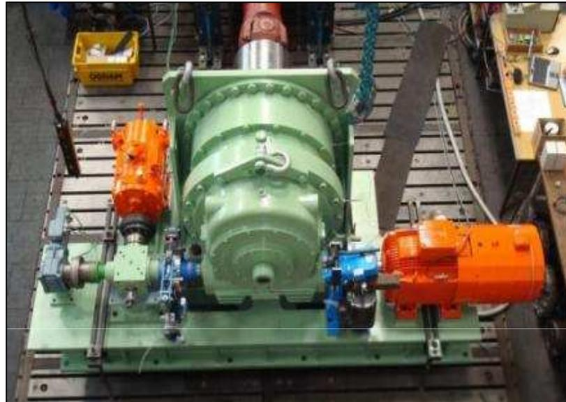
Drive Unit for 400 t Drum Type Furnace
